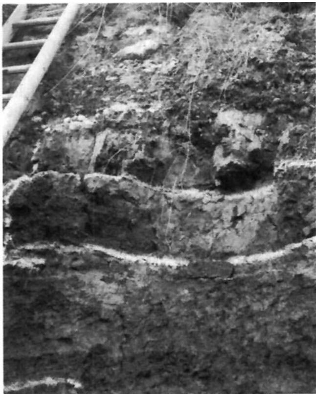
Image 3: Suspected solifluction surface in a post-failure test pit. Source: Rowe (1991).
