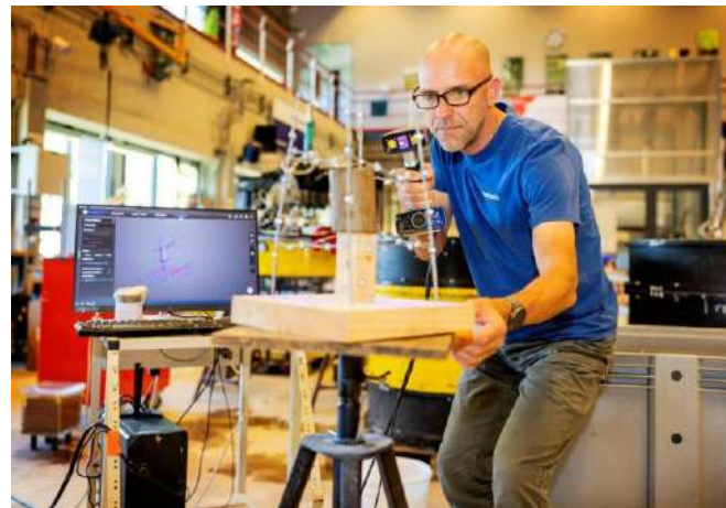
Remco van den Berg, project engineer, is measuring volumetric changes of a clay sample through 3D scanning.
